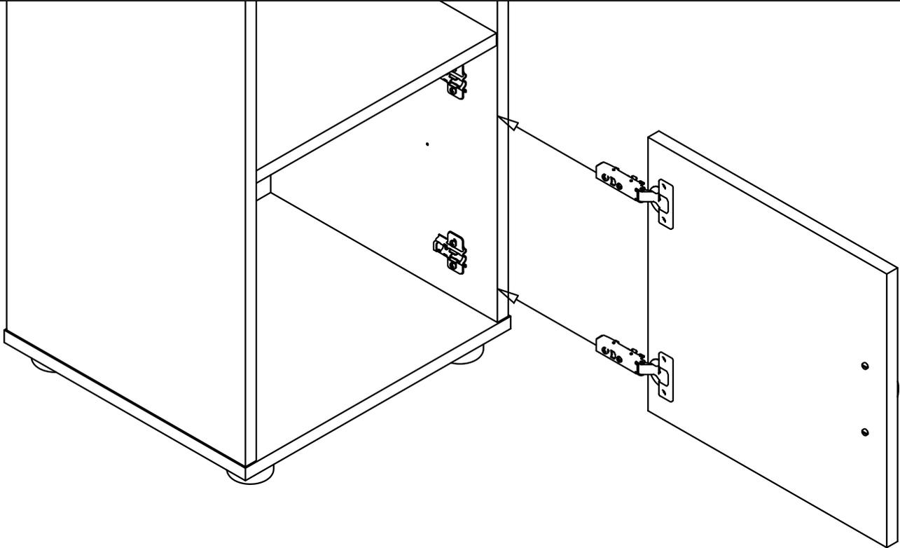
Ensure the hook of the hinge locates into the hinge plate.
