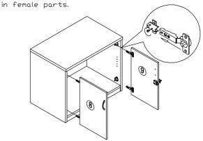
13 Install Door Hinge female parts onto side panels.
