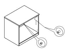
16. Install doors onto cabinet by sliding door hinge male parts into its female parts and fasten the screws
