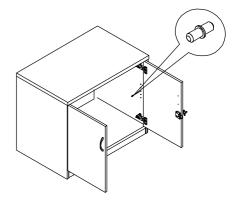
14 Install Lock in Right Door, Door Catch in Left Door and Door Hinge male parts in Right/Left Doors.
