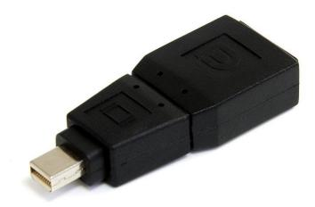
The GCMDP2DPMF Mini DisplayPort to DisplayPort adapter/converter allows you to add a standard DisplayPort connection port to your existing laptop or Mac® Mini. Easy to use and install, this cost-effective solution makes it easy for you to go from Mini DP to DP, in order to get the most from your Mini DisplayPort device.
