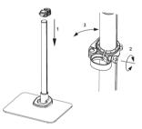
4. Slide the Iron Position Ring (5) onto the Cable Clip (4), with the flanges facing upward.
