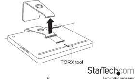
7. Align the hole in the Flange (7) with the pin on the back of your iMac, then use the Torx Tool (12) and the screws removed in the previous step to attach the Flange.
