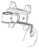
To increase / decrease swivel resistance, adjust the set screw located on the side of the Monitor Mount bracket at the Support Post, using the 3mm Allen Wrench (10).
