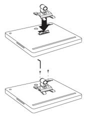
10. Slide the Monitor Mount (3) onto the Support Post (2) until it rests on the Iron Position Ring (5) and tighten the set screw using the M3 Allen Wrench (15).
