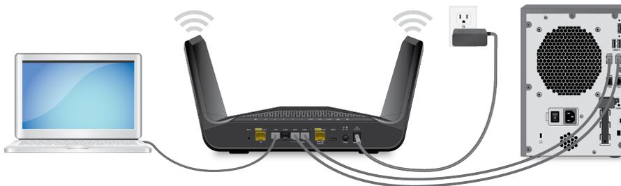
Figure 8. Ethernet port aggregation to a LAN device
