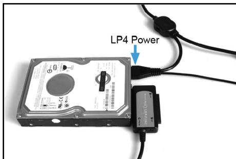
Connecting the LP4 Power Connector
