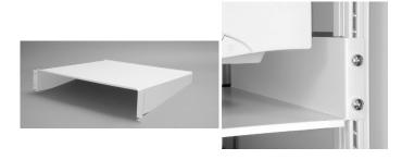
2. Deep Shelf - Before installing the deep shelf into the cabinet you must first join the mounting bracket to the shelf using the screws and nuts provided. Move the nuts in the cabinet to the desired hight and fasten the shelf's brackets to the front and rear posts.
