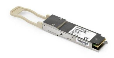
The QSFP40GESR4E is a Dell EMC QSFP-40G-ESR4 compatible fiber transceiver module that has been designed, programmed and tested to work with Dell EMC brand switches and routers. It delivers dependable 40 GbE connectivity over fiber cable, for 40GBase-SR4 compliant networks, with a maximum distance of up to 400 m (1312 ft.).
