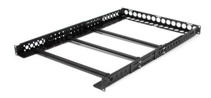
These 1U server-rack rails let you mount non-rackmount equipment such as desktop servers, networking equipment or KVM switches, into your 19" server rack without sacrificing 1U of rack space, like you would with a traditional shelf. The rack rails are also a great solution for mounting equipment with damaged rails or discontinued OEM equipment such as  $Dell^{TM}$ , IBM@, HP@ or Apple servers that no longer have rack rails available.
