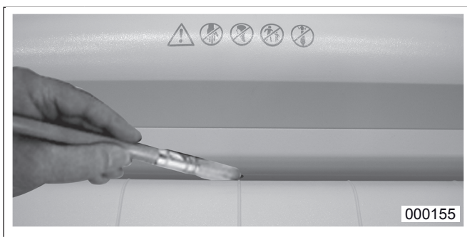
fig.7 Cleaning the photocells
