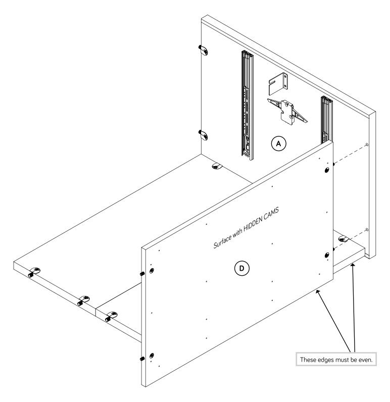
Fasten the LEFT END (B) to the BOTTOM (D) and BACKS (G). Tighten two HIDDEN CAMS and tighten four TWIST-LOCK® FASTENERS.
