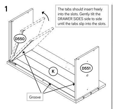
Insert the DRAWER SIDES (D550 and D551) at an angle into the slot at each end of the SMALL DRAWER FRONT (K).
