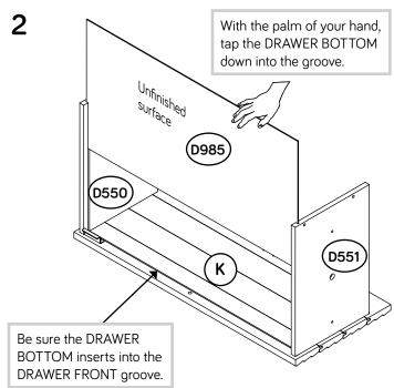
Slide the DRAWER BOTTOM (D985) into the grooves in the DRAWER SIDES (D550 and D551) and SMALL DRAWER FRONT (K).
