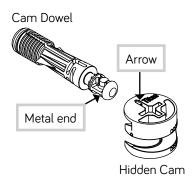
Push a HIDDEN CAM into the part. The arrow in the HIDDEN CAM must point toward the hole in the edge of the board.
