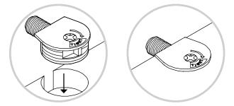
2. 1. Insert the dowel end of the FASTENER into the hole of the adjoining part.
